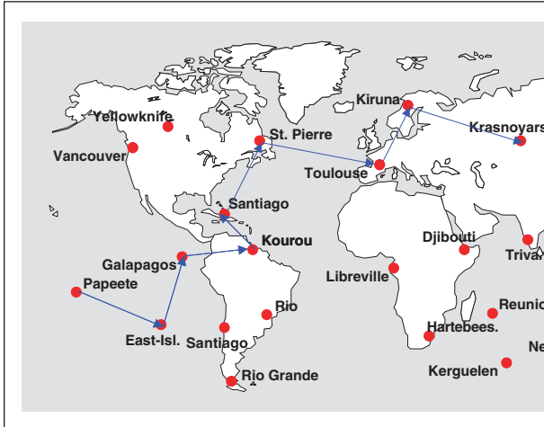
Fig. 4. Example of linked common-view time transfer.
